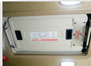
Two Emergency Exit Roof Hatches
