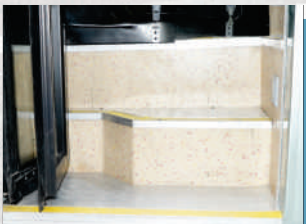
Low Footstep for Easy Entry/Exit with Driver Controlled Door
